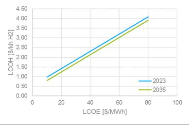
LCOH in function of LCOE for 2023 and 2035.
