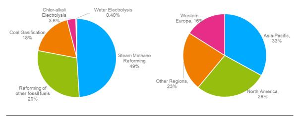
Left.: Global production of Hydrogen by source. Right: Global production of Hydrogen by region.
