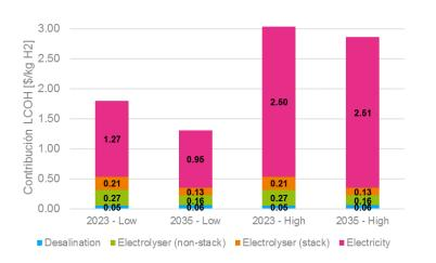
Contribution of the upstream building blocks of the hydrogen value chain for LCO<sub>High</sub> and LCOH<sub>Low</sub> in 2023 and 2035.
