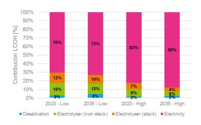
Contribution of the upstream building blocks of the hydrogen value chain for LCO<sub>High</sub> and LCOH<sub>Low</sub> in 2023 and 2035.
