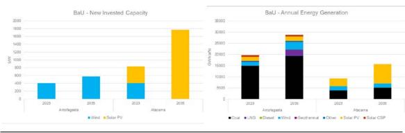
New invested capacity and energy generation for the BaU scenario for Antofagasta and Atacama.
